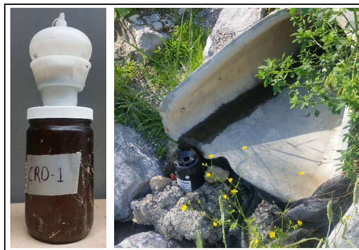
Figure 5: left—first flush jar; right—housing in rock apron
